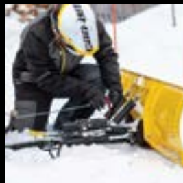
Attach the winch cable to the plow using a guiding hook/roller.
