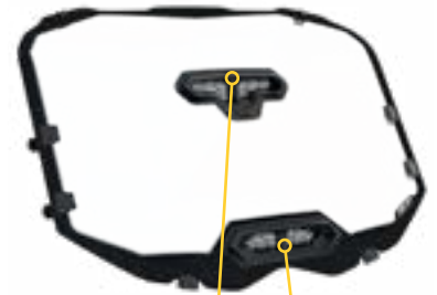
Upper vent channels air into the cabin
