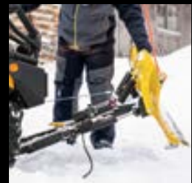
Remove the winch cable from the guide. You're ready to plow.
